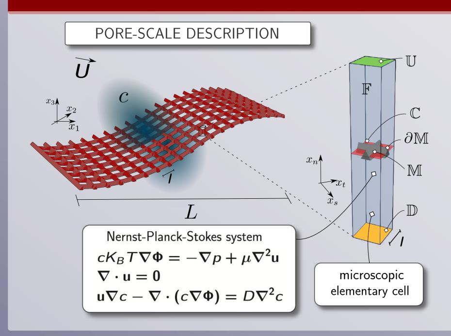
Osmotic flow of a solvent of density ho and viscosity  $\mu$  and a solute of diffusivity D through a thin porous structure of chemical potential  $K_B T \Phi$  via the Nernst-Planck-Stokes system. Homogenization works like a selective magnification lens and provides interface conditions valid on a fictitious macroscopic membrane  $\mathbb{C}$ .
